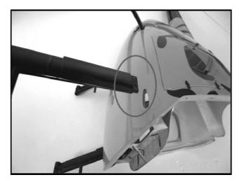
4.3 Insert the skids into the struts as shown.
