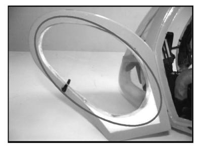
4.17 Glue in the tail window with epoxy resin adhesive.
