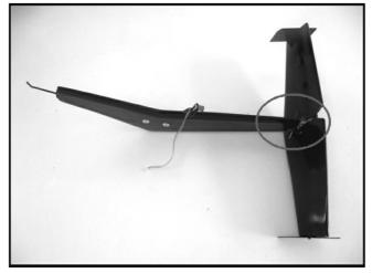
4.19 Screw the tail unit with M3x12 and washer M3.
