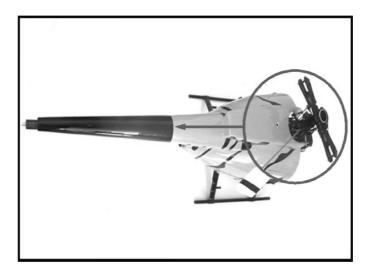
4.10 Ensure that the tail linkage exits as shown.
