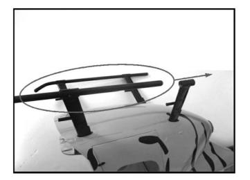
4.4 Secure the skids with 4 set screws M3x4 as shown.
