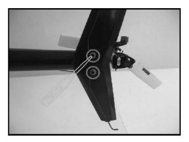
4.20 Secure the canopy with screw M3x12 and washer M3. Do not fly without securing the canopy with this screw. It will fall off.
