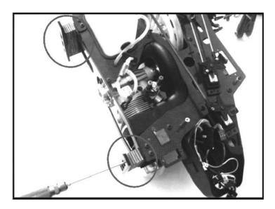
4.9 Insert the mechanism into the fuselage as shown.
