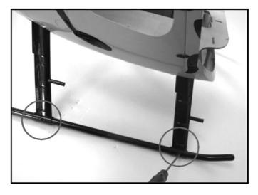
4.5 Fix the struts with 4 screws M3x12 as shown.
