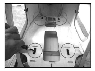
4.6 Assemble the tail bracing as shown.
