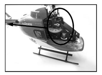
4.9. The wooden adapters must be inserted into the detent.
