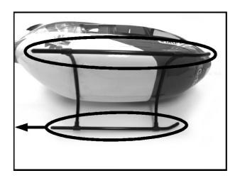
4.4. Attach the step plates using 4 pieces of Screw A2x10 as shown.
