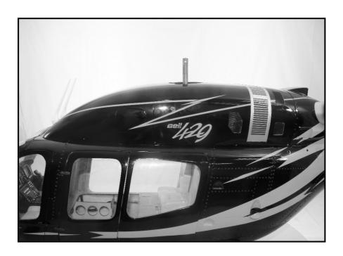
4.22. Finally glue all scale parts (14-18) as shown into the fuselage.
