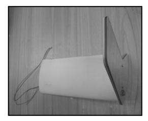
4.19. Glue the tail units carefully into the tail boom using epoxide glue. Secure them with tape while the adhesive cures. Align them carefully.
