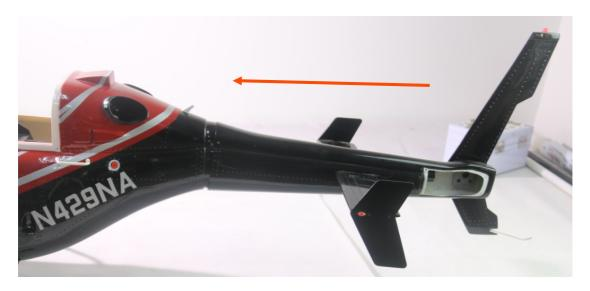
4.15. Attach the supplied L-Lever (27) onto the tail rotor unit as shown. Then attach onto the tail boom, tighten screws and attach all linkages.
