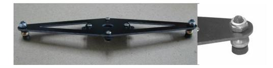
4.11. Mount the servo as shown in the wooden frame. Then mount the horn and prepared lever onto the servo. Use the pushrods with the ball link ends to connec the servo lever with the levers on the retract shafts as shown. Do not tighten the screws on the retract shaft levers yet.
