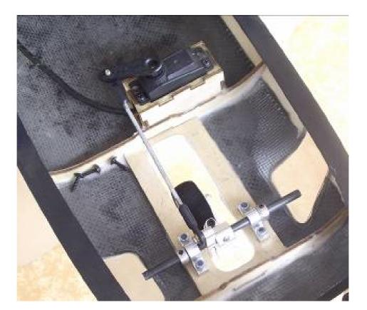
4.7. Insert carbon rods 3x45 as shown.
