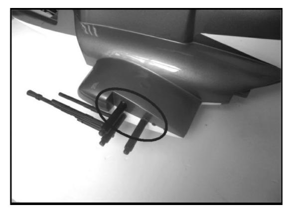
4.23. Then use glue to attach the end plate on both sides. Match the painting of the fuselage!
