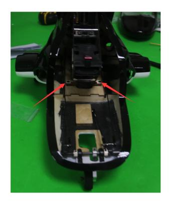
4.15. The screw down the tail section from below as shown.
